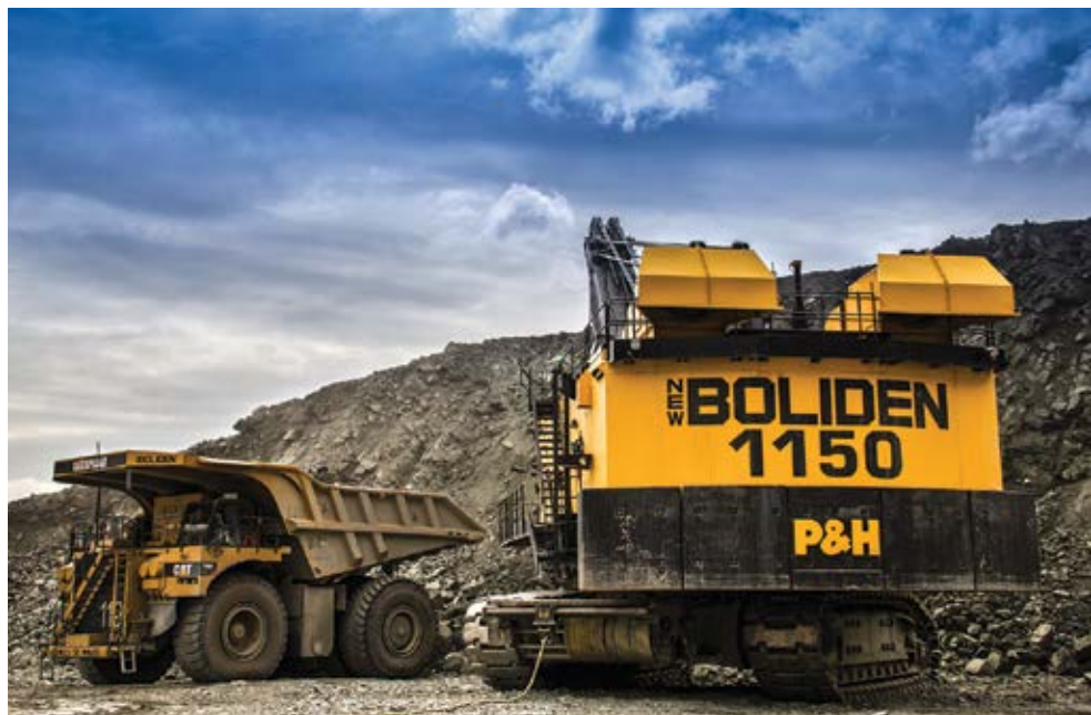
A rope-shovel loads ore into a haul truck at Boliden's Aitik mine. (Photo: Lars deWall)
