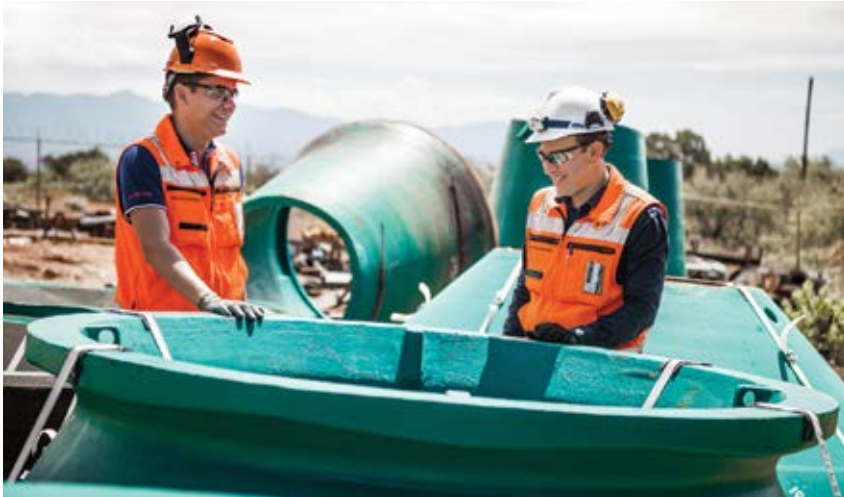
Experts examine crusher wear parts as part of a chamber optimization program. (Photo: Metso Outotec)
