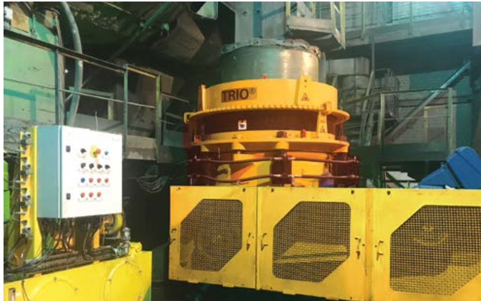
The team at Weir recently supplies custom-engineered ESCO crusher liners to an iron-ore mine in Russia. The customer gains four more days of wear life with a 16% increase in the bowl liner life and a 20% increase in mantle utilization. (Photo: Weir Minerals)
