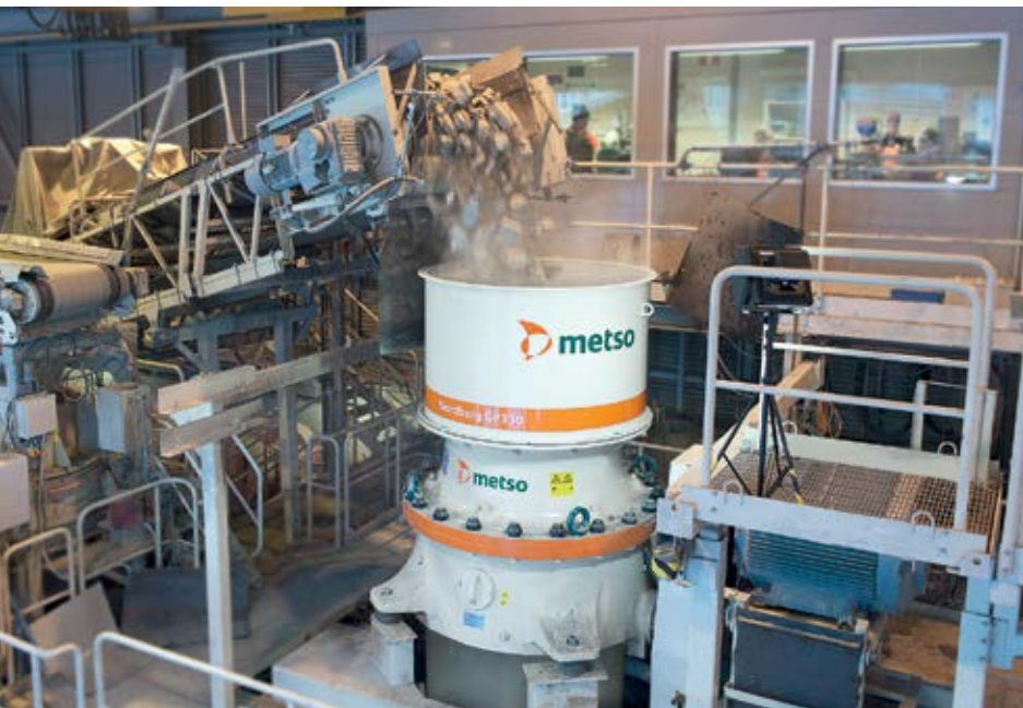
A Metso Outotec Nordberg GP330 cone crusher in operation. (Photo: Metso Outotec)
