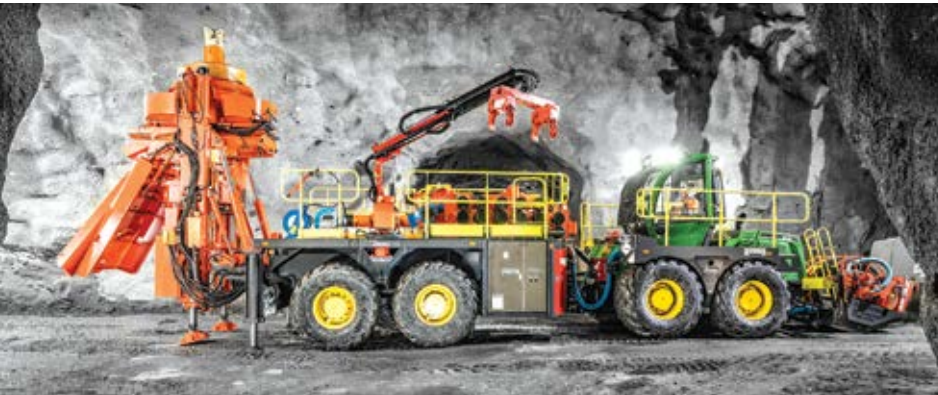
Nimble and manageable by one operator, the Rhino 100 inspires a revolution in thinking about production drilling. With record-breaking speed, it can raise bore slot raises to serve as void spaces for blasting for improved fragmentation and the many downstream benefits. (Photo: Sandvik)
