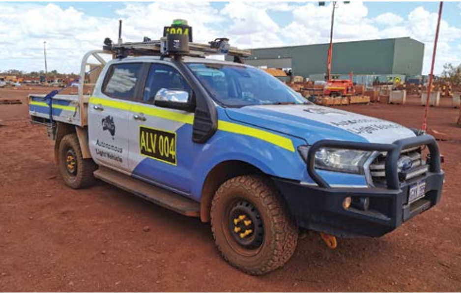
Four Ford Rangers were retrofitted with an on-board vehicle automation system to support a driverless equipment transfer service.
