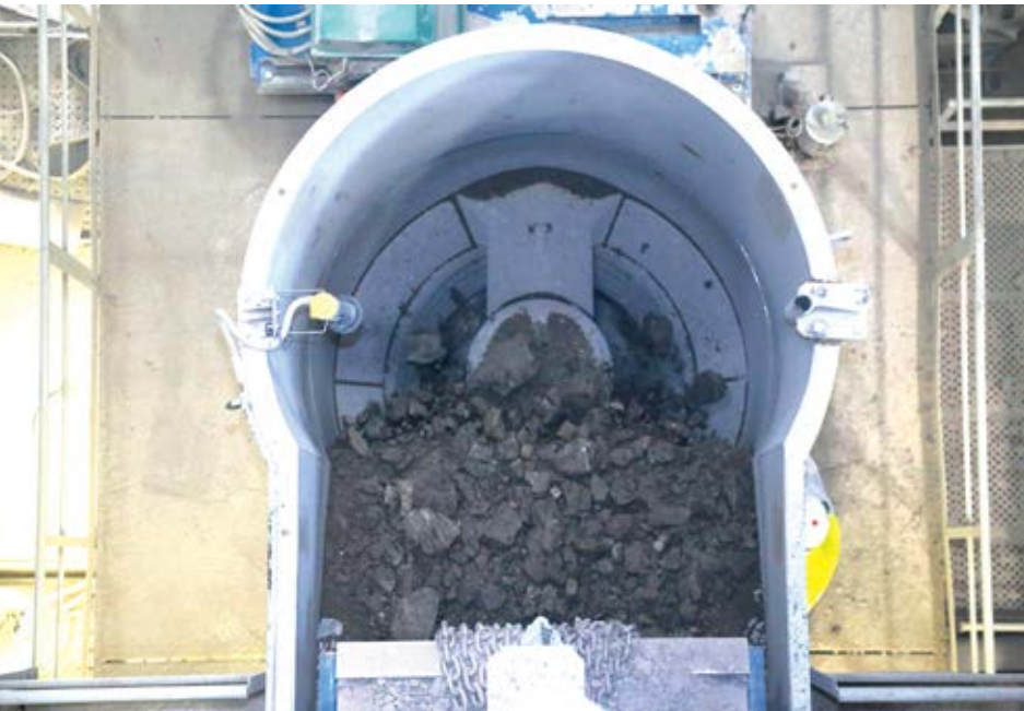
Cone crushing often provides the most economic and reliable method for secondary crushing in mineral processing applications. (Photo: thyssenkrupp)
