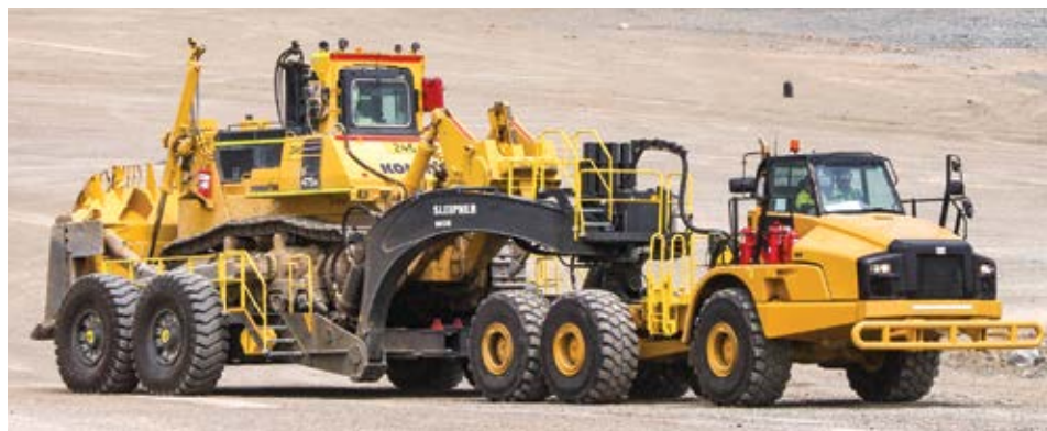
The DB120 has a maximum payload of 120 mt and a maximum towing speed of 15 km/h fully loaded, and can be towed by a 45-mt ADT. (Photo: Sleipner Finland Oy)
