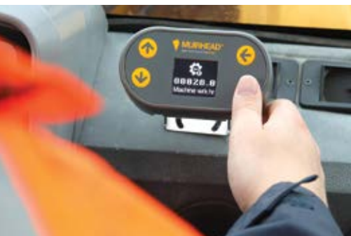
RCT's vehicle-mounted Smart Service Monitor alerts operators and maintenance personnel to an upcoming need for service, based on user-selectable parameters.
