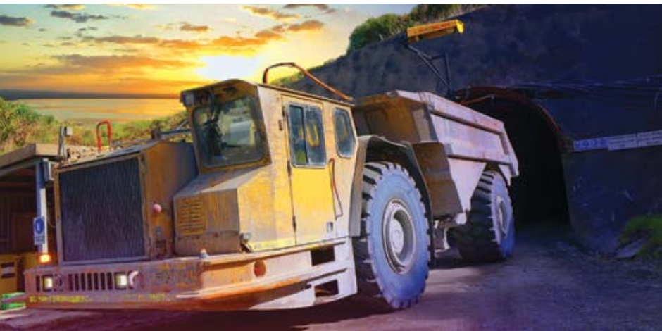
Underground mining truck passing under a Loadscan LVS system in New Zealand.
