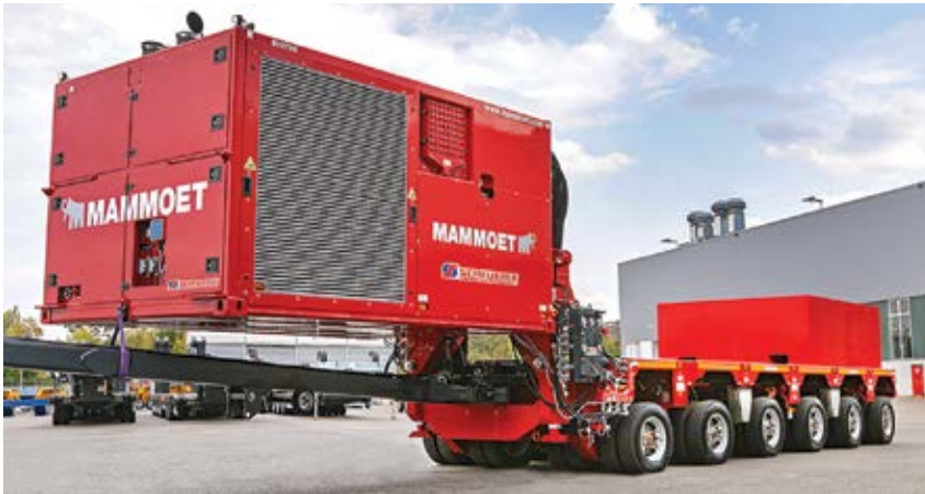
Trailer Power Assist, co-developed by SCHEUERLE and Mammoet is based on the self-propelled K25 modular platform vehicle, drives four of six axle lines, and is situated between a truck and a trailer to provide additional traction force of 400 kilonewtons. (Photo: SCHEUERLE)
