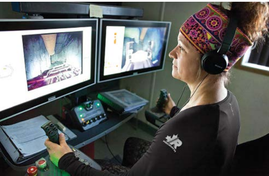
Using the latest technology, a Redpath miner operates an LHD from the surface using teleremote controls.
