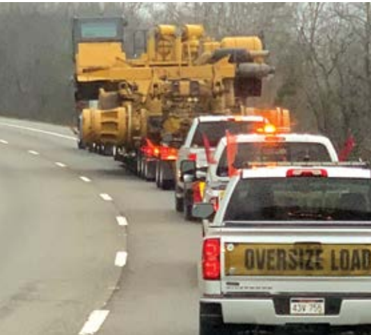
JP Tech Services used its own certified escorts to accompany the 10-axle rig hauling a 785C chassis on another gray West Virginia Sunday in late fall. (Photo: JP Tech Services)
