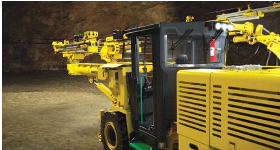
Komatsu's new ZJ21 jumbo drill rig and ZB21 bolting rig feature a boom design that permits swapping of a drill feed system for a bolting setup and vice versa. The machines are based on a common platform that optimizes operator familiarity, maintenance efficiency and parts inventory requirements.
