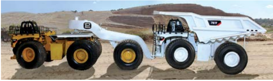
The Vehicle Recovery Tool attaches to the towing machine to boost capacity, provide greater stability and balance, and improve safety. (Photo: PHIL)
