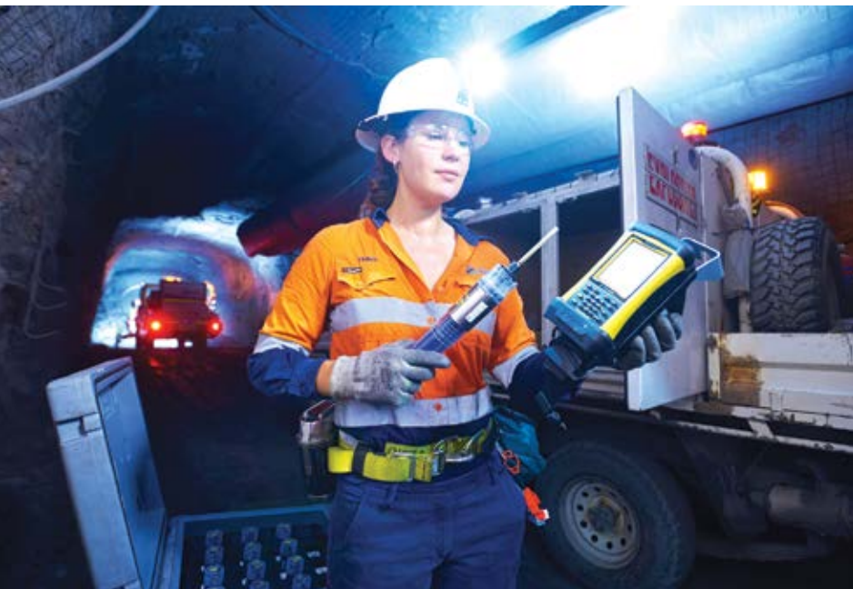
Orica's wireless initiating system technology, WebGen, in use at Glencore's Ernest Henry mine. (Photo: Orica)
