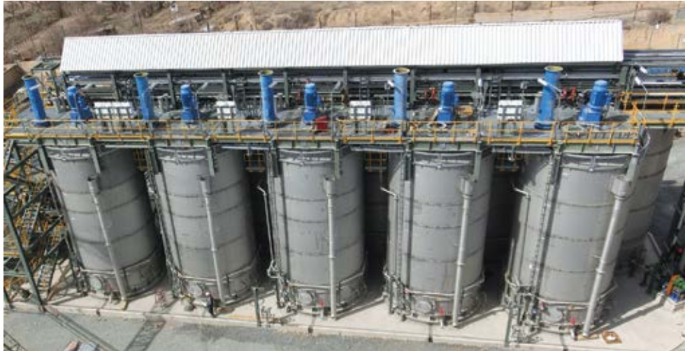
A lab in Randburg, South Africa, will qualify operations for Albion Process. The process is a combination of ultrafine grinding and oxidative leaching. (Photo: Liebherr)
