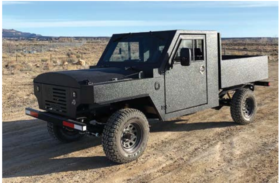
The Small Boss Buggy features a Tier 4-Final engine with streamlined electronics. To facilitate maintenance and cut costs, it has neither a diesel particulate filter nor diesel exhaust fluid. (Photo: Genco)
