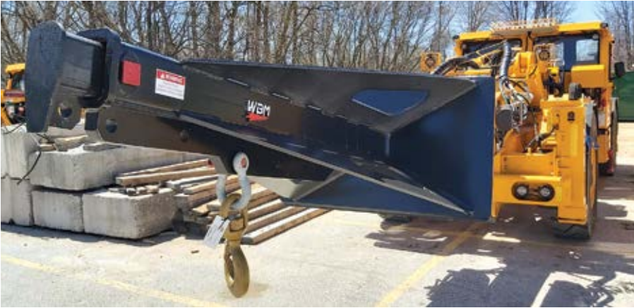
The jib boom attachment for the LR3 has a 7,000-kg load capacity and can be used to pull pumps from sumps. (Photo: MacLean)
