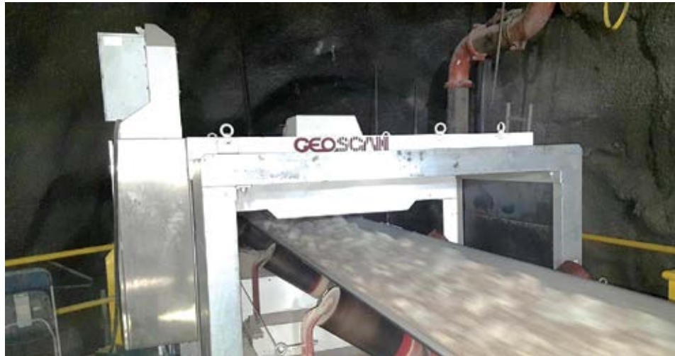
The GEOSCAN-M analyzer installed on an underground conveyor belt at the New Afton mine for bulk sorting of Cu-Au ore from the block cave. (Photo: Scantech International)
