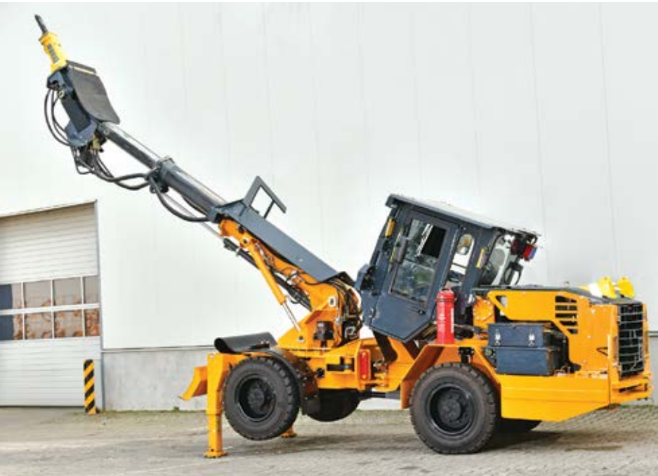
The compact PScale 8-T precision scaler was designed to give operators more control over where and how to scale. Developed in Peru, it can handle heavy use in extreme environments. (Photo: Paus)
