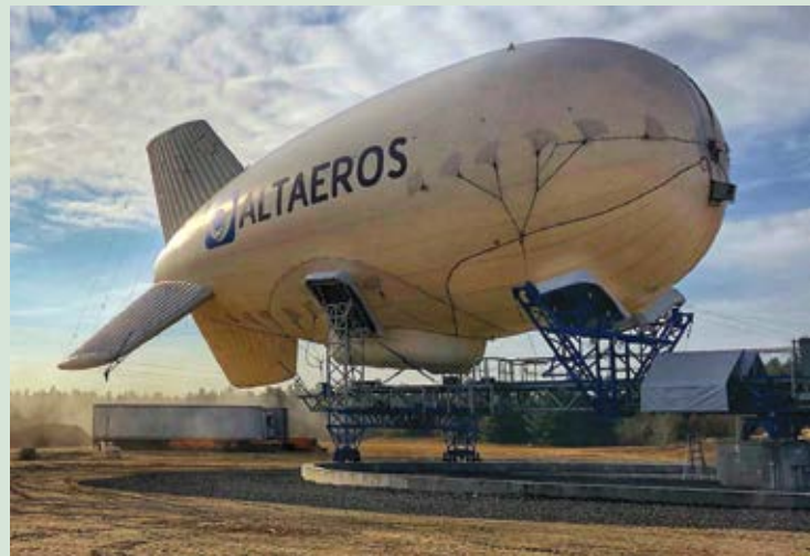
Altaeros' SuperTowers are autonomous, tethered aerostats that can lift wireless payloads up to 300 m into the air to provide wide-area coverage at mine sites. (Photo: Altaeros)
