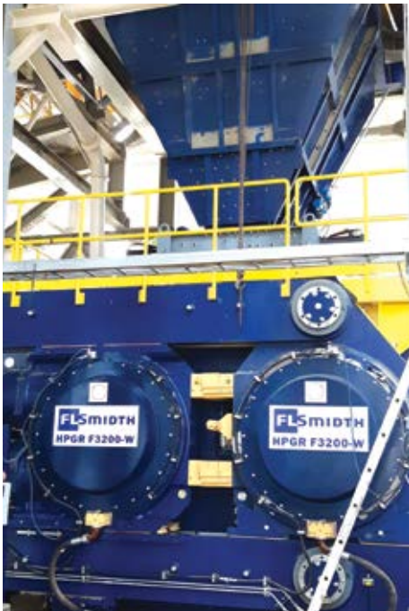
HPGRs gain traction in copper thanks to their ability to significantly reduce energy consumption at the front end of flowsheets. (Photo: FLSmidth)
