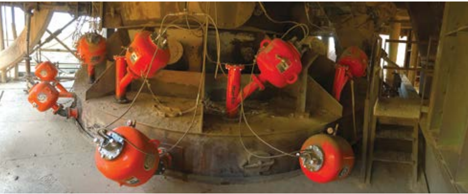
Air cannons can be useful in preventing troublesome material accumulation in process equipment, minimizing the need for downtime and manual labor.
