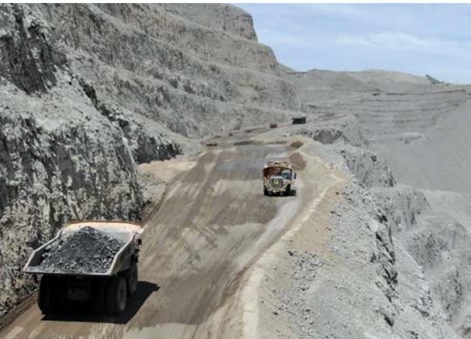
The Candelaria open-pit mine moves 270,000 metric tons per day (mt/d) of which 43,700 mt/d is copper ore.
