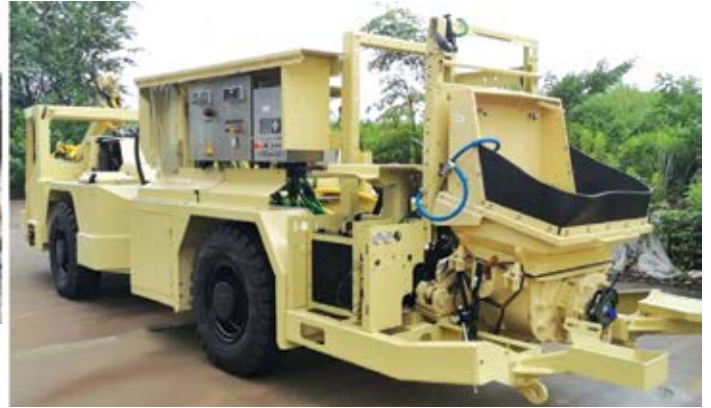
Normet's reman program offers on-site rebuilds, and can help isolated mines maintain the needed equipment availability even when under tight travel and transportation restrictions. (Photo: Normet)
