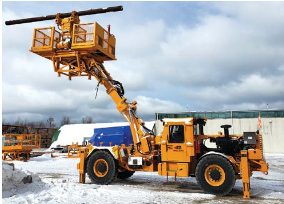
The latest utility equipment releases give operators more control and operations more options. Above, MacLean's new pipe handler basket for the LR3 integrated carrier can be attached quickly, and can transport, lift and rotate pipes. (Photo: MacLean Engineering)
