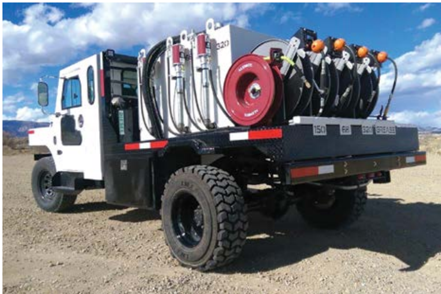
With a Tier 4-Final Engine, the HD Series Lube Truck has four wheel drive, straight tube axles and dual-piston hydraulic steering. (Photo: Genco)
