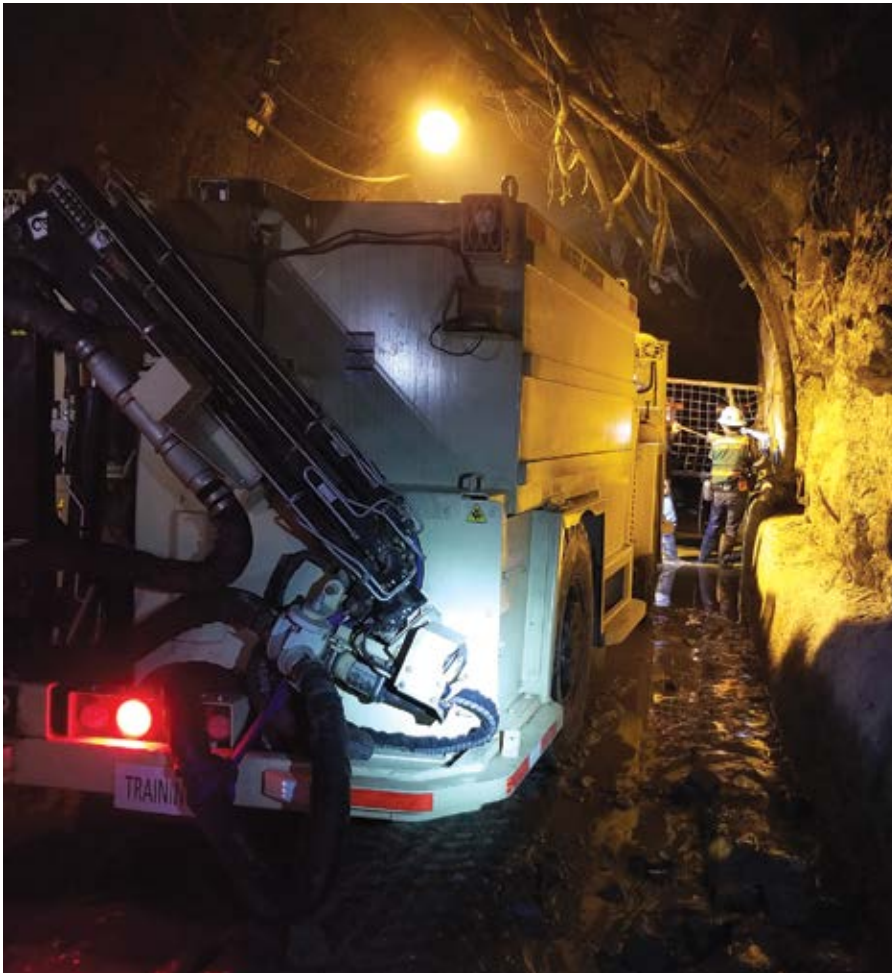
The A64 HD Water Cannon made short work of clearing drawpoints and previously backfilled ore passes at a block caving operation. (Photo: Getman Corp.)
