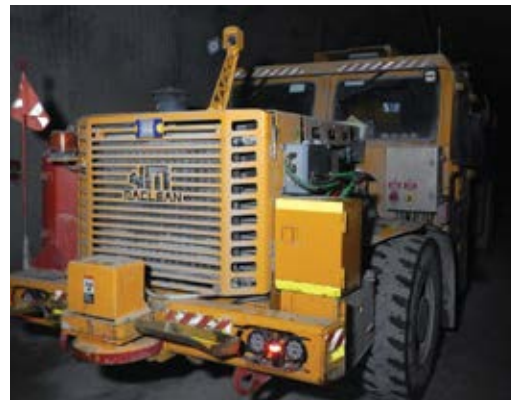
At Cadia Valley, a MacLean water cannon is integrated with Epiroc's traffic management system so the unit could be teleoperated from the surface. (Photo: Newcrest Mining)
