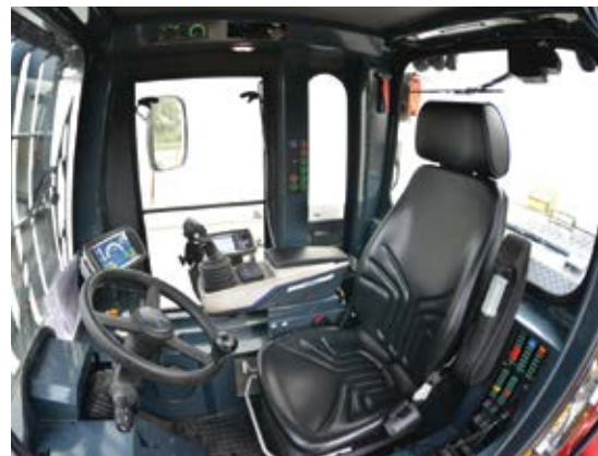
Tilted at up to 20°, the cabin for the PScale 8-T cuts noise, vibration and heat, and offers excellent visibility. (Photo: Paus)
