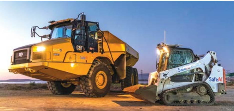
SafeAI retrofits heavy equipment for autonomous applications in both mining and construction. It's platform currently supports trucks from 30-ton ADTs to 220t rigid-frame haul trucks, as well as dozers and skidsteers. (Photo: SafeAI)
