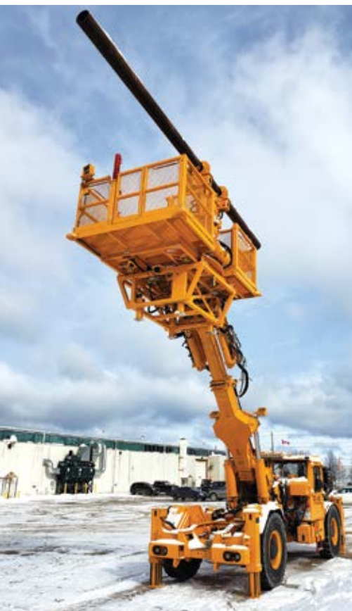
The new pipe handler basket for the LR3 integrated tool carrier has adjustable claws, a tilting grapple feature, 240° basket rotation, dual control stations and the ability to store pipes. (Photo: MacLean)
