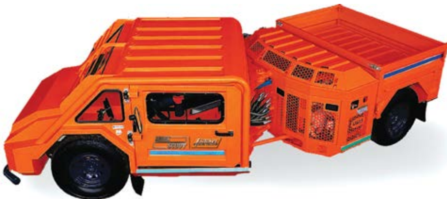
The Mine Scout is developed to safely speed technicians from underground to surface worksites at mines in Africa. (Photo: J.H. Fletcher)
