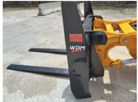
The fork attachment for the LR3 has a 6,350-kg load capacity and can be used to load ventilation fans into cradles. (Photo: MacLean)
