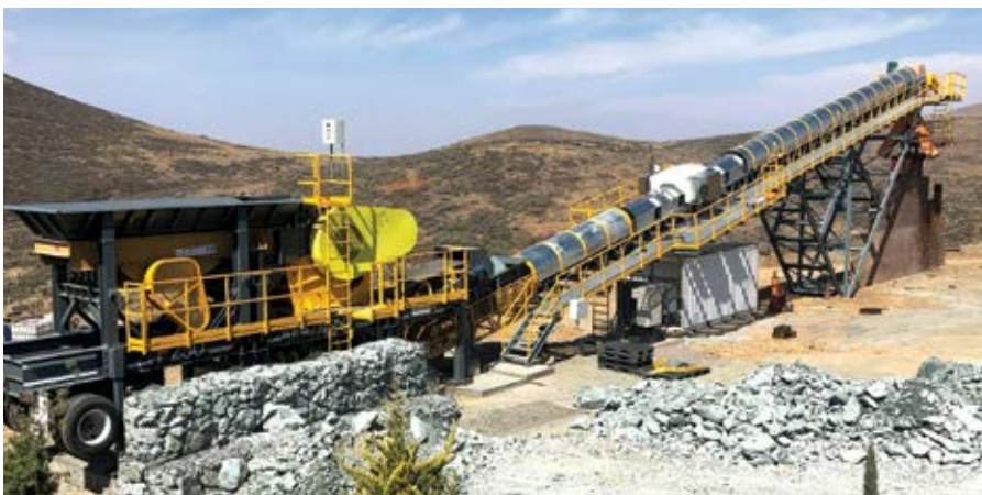
Capstone Mining’s Cozamin polymetallic mine in Mexico opts for a 200-mt/h bulk sorter from NextOre to upgrade the copper domain within its orebody. (Photo: NextOre)
