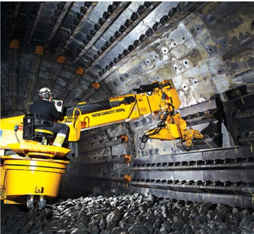
The AG mills for Boliden's Aitik copper mine use Metso Outotec's Megaliner mill lining. (Photo: Metso Outotec)
