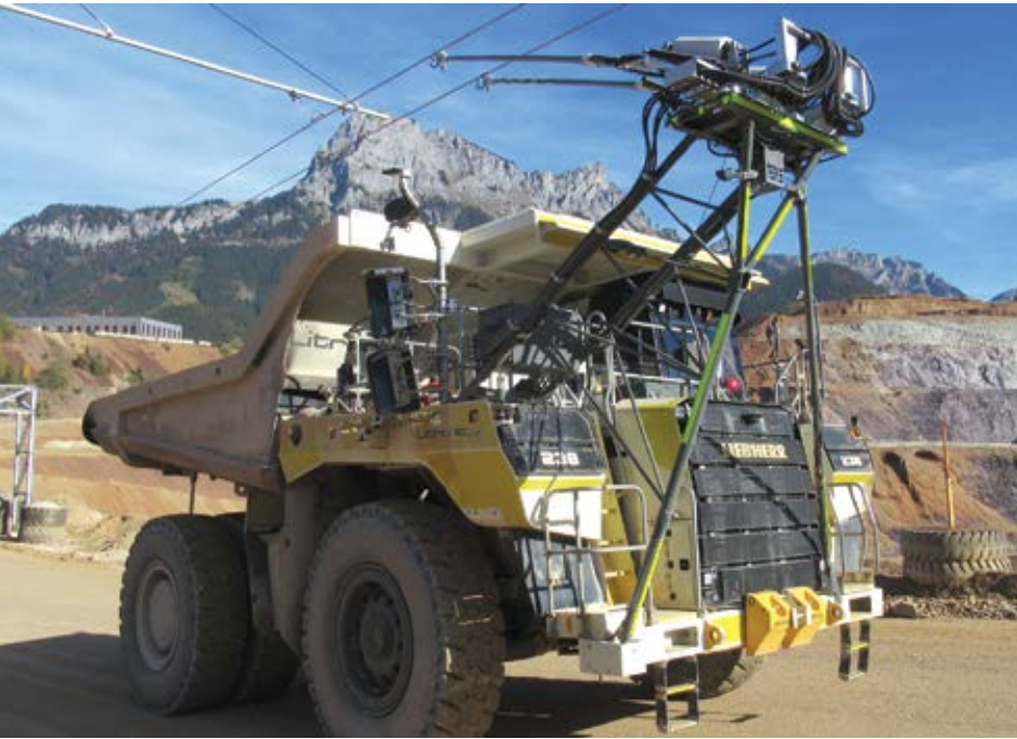
A trolley system using overhead lines was tested at an iron ore mine in Austria. The system allows for switchbacks. (Photo: Liebherr)
