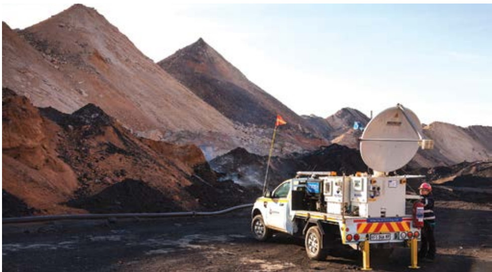
Reutech Mining’s MSR Modular series models can be truck-mounted, can integrate other sensors and third-party solutions, and can operate in extreme environments. Above, a unit scans for submillimeter movement at Landau coal mine in Mpumalanga, South Africa. (Photo: Reutech Mining)
