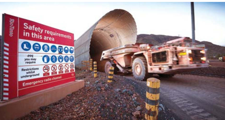
An LHD exits the Argyle mine portal, which can trace its roots back 37 years.
