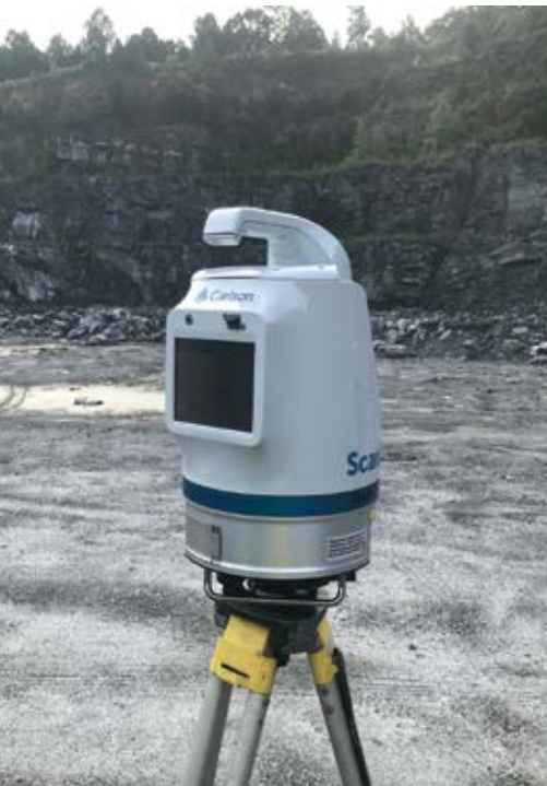
Equipped with a camera, inclinometers, and a LIGNSS receiver, Scan2K can be wired for power and data, or can operate on a battery and wireless. It can be controlled by third party slope stability software. (Photo: Carlson Software)
