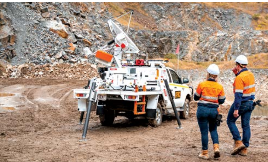
GroundProbe’s SSR-Agilis is mounted on a light vehicle for easy relocation, and can sit anywhere from 30 m to 1,400 m from the target. It has an integrated camera, making it easier for users to locate movement detected by radar. (Photo: GroundProbe)
