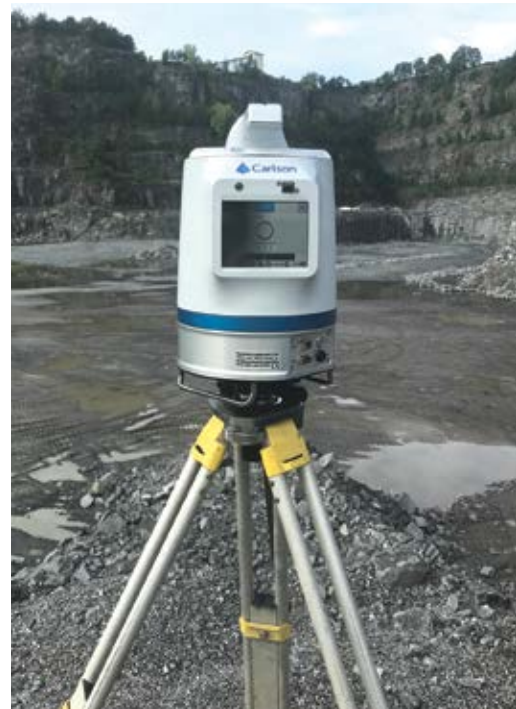
The Scan2K is designed to fill the gap between smaller short-range scanners and bigger long-range scanners. Unlike other LIDAR scanners, Scan2K can operate in mines that use prisms in slope monitoring. (Photo: Carlson Software)
