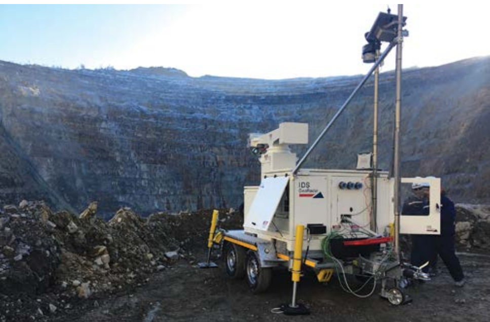
Recent updates allow Hexagon's HxGN Collision Avoidance System and IDS GeoRadar's IBIS Guardian to communicate directly for speedy slope stability alerts and the rapid creation of geofenced no-go zones. Above, an IDS GeoRadar unit scans a shadowy distant slope. (Photo: Hexagon Mining)
