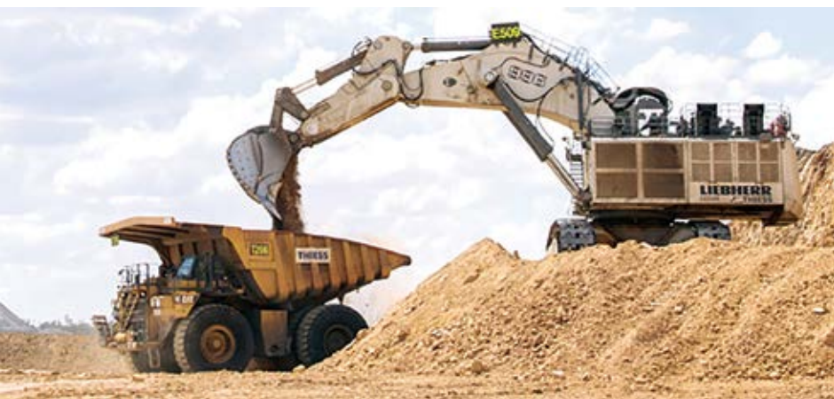
Thiess will continue to operate and maintain three 600-mt excavator fleets at the Caval Ridge mine (above) to move additional overburden. (Photo: BMA)
