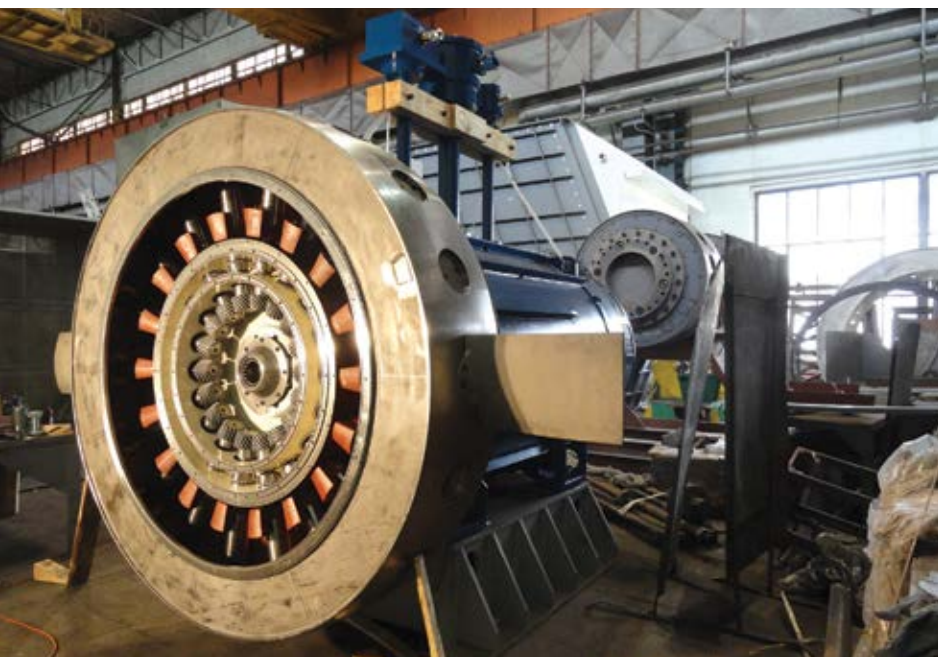
For CFE's flagship axial fan system, with push-button reverse capability, the impeller assembly is mounted on a shaft end from the main motor. An actuator on the impeller hub then controls the blades in flight. (Photo: CFE)
