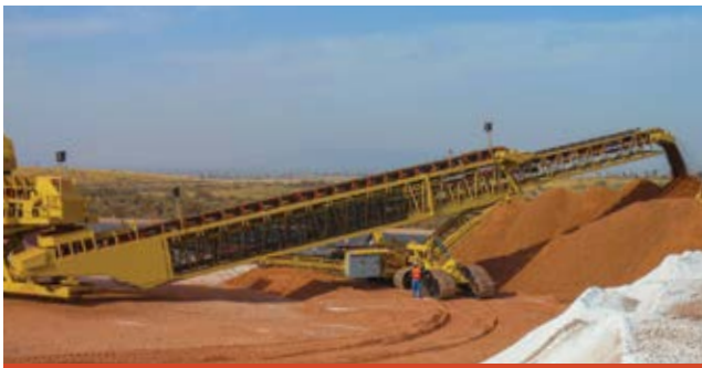
TELESTACKER® CONVEYOR PILES MORE MATERIAL PER MOVE
