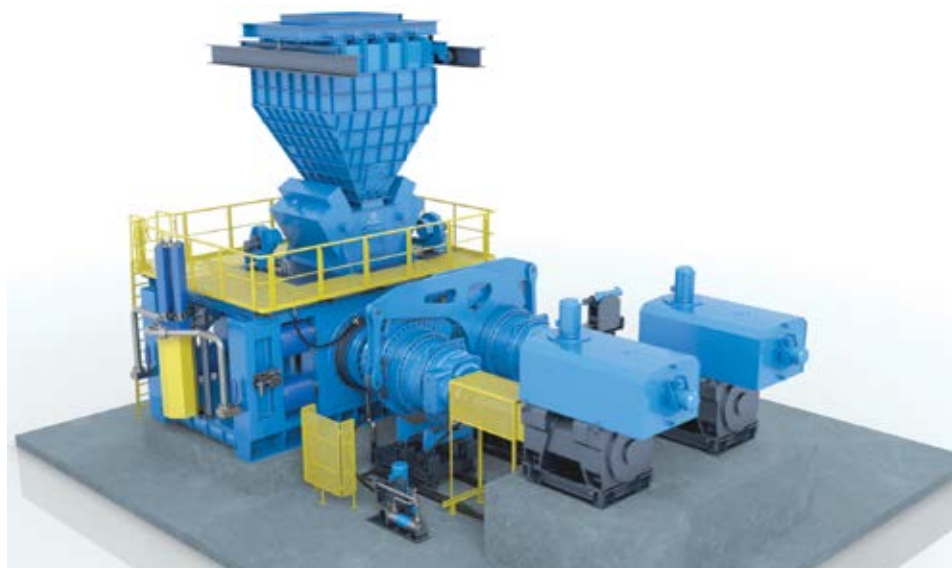
thyssenkrupp’s new HPGR Pro model uses rotating sideplates on the fixed grinding roll — a design innovation claimed to enable improved material feed and up to 20% more throughput compared with conventional HPGR designs.
