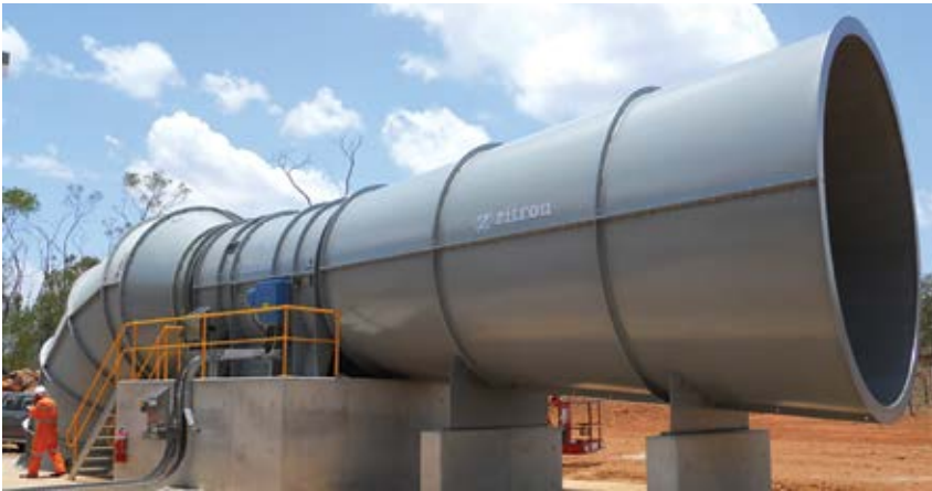
In 2012, Zitrón S.A. installs the 630-kW ZVN 1-30-630/8 fan system at Pajingo gold mine in Queensland, Australia. (Photo: Zitrón S.A.)
