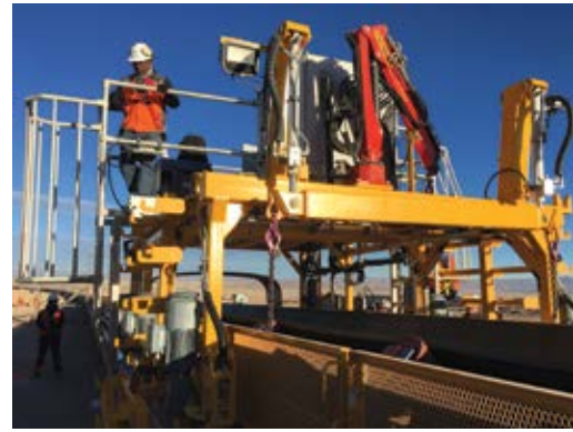
To replace idlers, a specially designed maintenance vehicle travels along the conveyor path.
