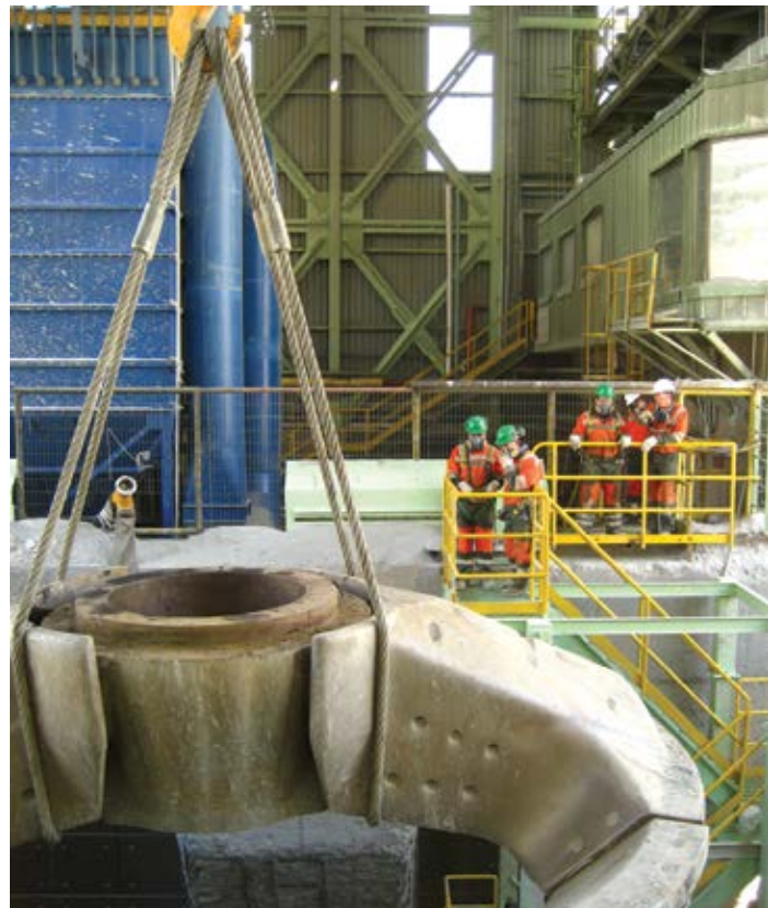
Maintenance under way on the primary crusher at Anglo American’s Los Bronces operation in Chile. (Photo: Metso Outotec)
