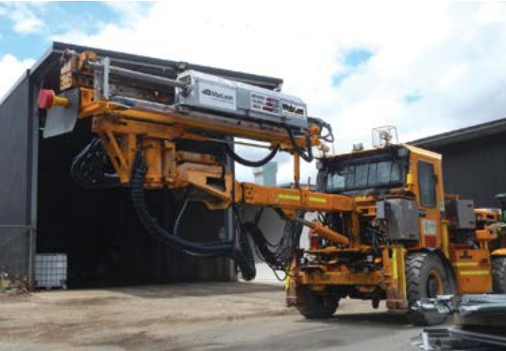
Above, Cadia's secondary break trial using MacLean's Auto Explosive Loader enabled with Orica's WebGen wireless technology. (Photo: MacLean Engineering)
