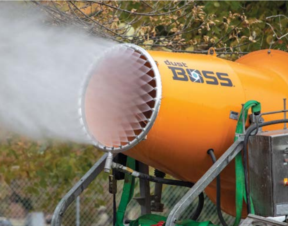
The line of DustBoss atomized-mist dust-control cannons produced by BossTek can be conveniently converted for use to broadcast Surface Disinfectant Cleaners (SDCs) for large-area sanitation purposes, according to the company.
