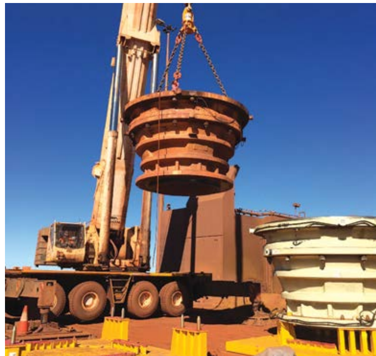
The new Metso rotatable top shell was developed at request from Australian mine operators who wanted a safer, easier to maintain design. (Photo: Metso Outotec)
