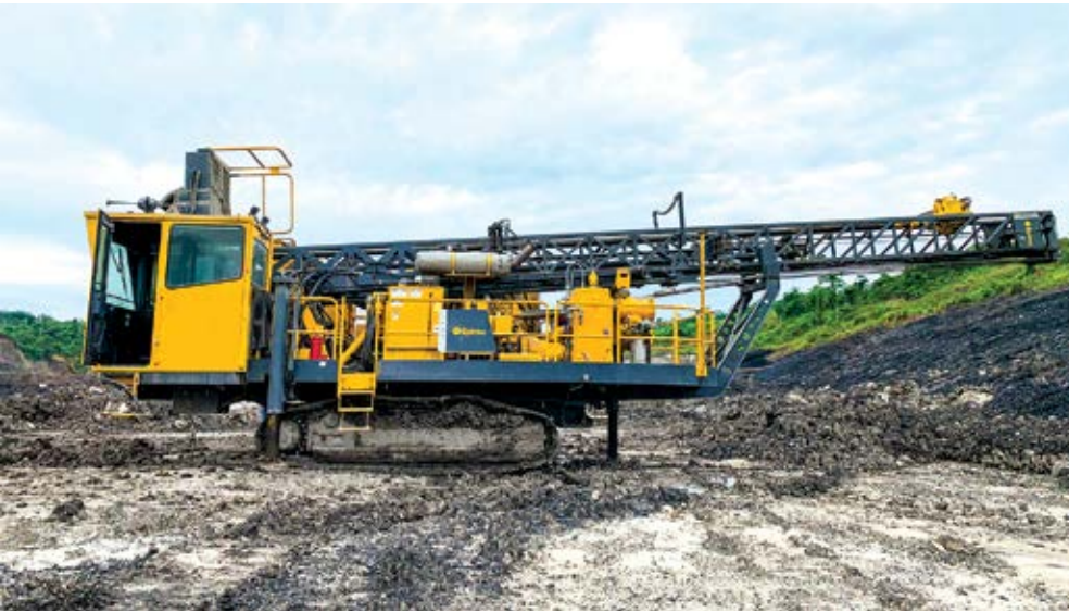
The DM30 II SP features an 11-m single-pass tower option that, Epiroc reports, increases productivity for 29- to 36-ft drilling conditions by eliminating the need to add a second drill steel. (Photo: Epiroc)
