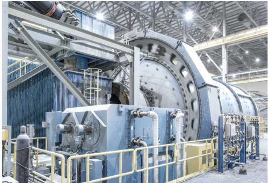
Zijin Mining's Veliki Krivelj adopted ABB dual pinion mill drives and other solutions that offer frozen charge detection, controlled roll back, automatic positioning, variable speed and cascade monitoring functionalities. (Photo: ABB)
