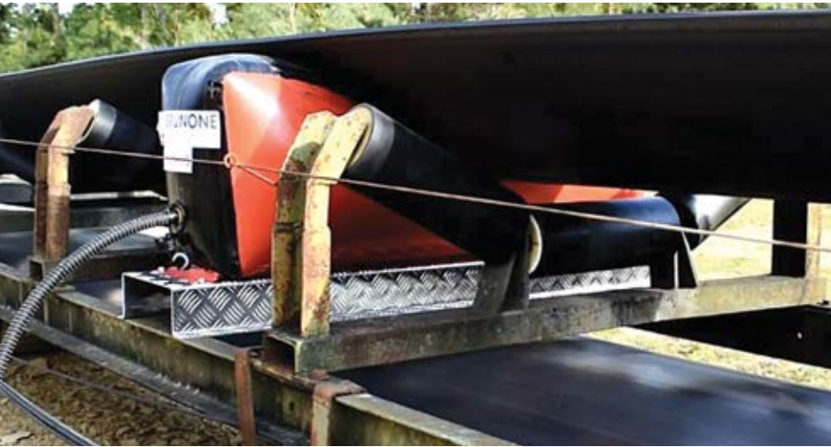
The Sparcric G developed by R. Brunone enables one worker to safely lift the belt for roller replacement.
