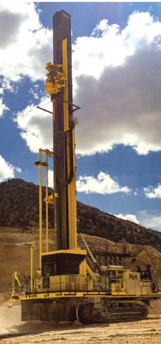
Field results suggest the P&H 77XR, released last fall, offers a reduction in maintenance costs of 5% to 10%, an increase in drilling time of as much as 12%, and an improved availability of 2% to 5%, Komatsu reports. (Photo: Komatsu)
