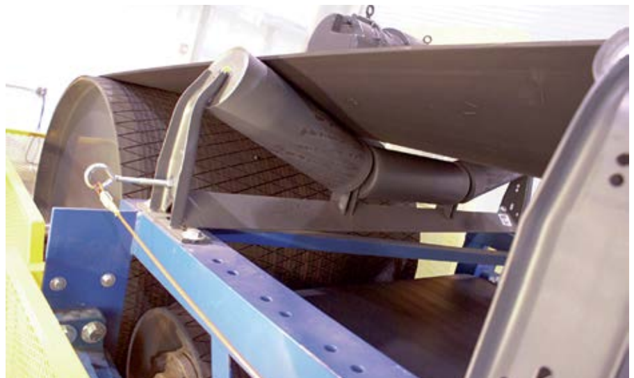
The pinch point between the belt and a carrying idler is one opportunity for an entrapment injury.
