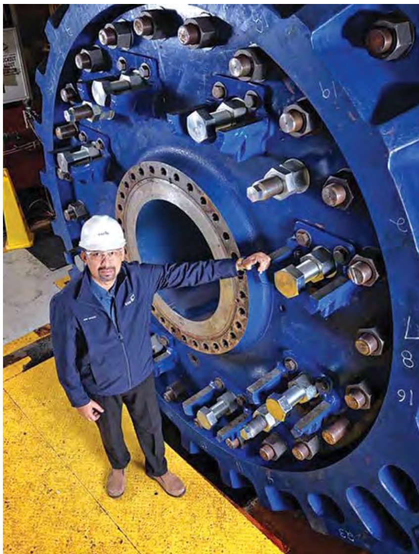
GIW Industries' TBC-92 slurry pump is the heavyweight king of the mining industry, according to the company, weighing roughly the same as a loaded medium-range, twin-engine commercial airliner.
