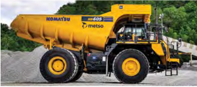
Two HD605-8 trucks with Metso bodies, described as up to 30% lighter than the OEM bodies they replaced, were delivered to a quarry in Belgium. (Photo: Metso)
