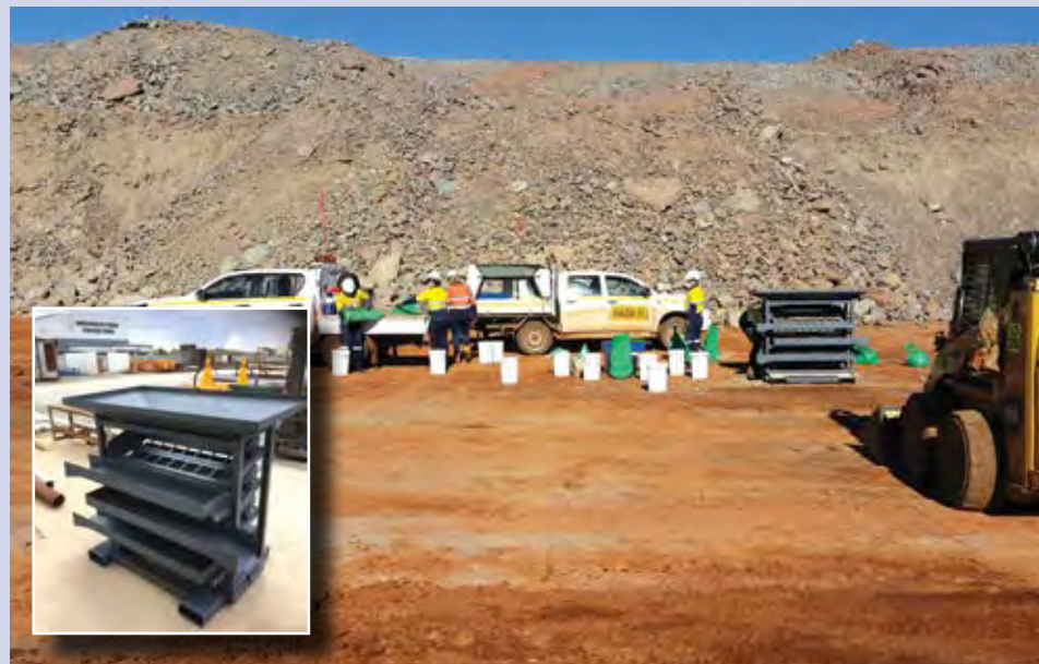
Using the ISPS screen deck, CRC ORE is conducting grade-by-size screening test work.
