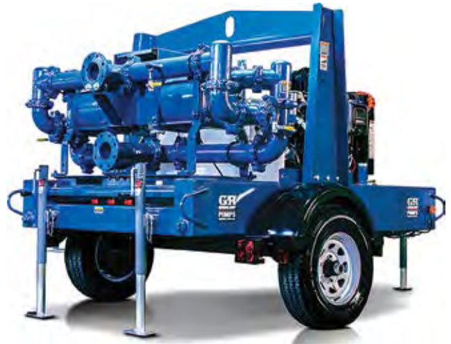
The highly portable Gorman-Rupp SludgeKat pump can handle slurries and sludges containing objects up to almost 2.5 in. diam, and can run for more than 24 hours on a full fuel tank.
