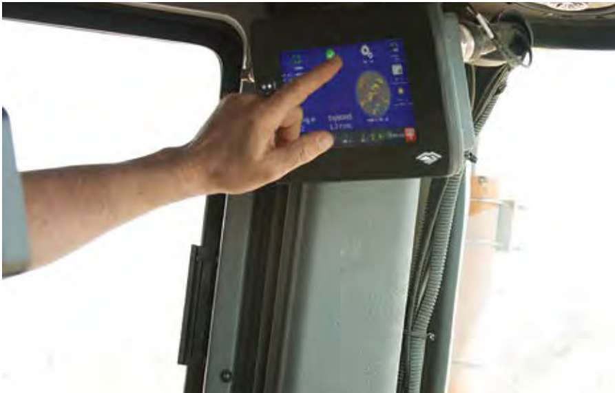
An in-cab display for Modular Mining's DISPATCH FMS. Today's systems must be capable of not only collecting the vast amounts of data generated by equipment on-board sensors, but also making the data relevant and actionable. (Photo: Modular Mining)
