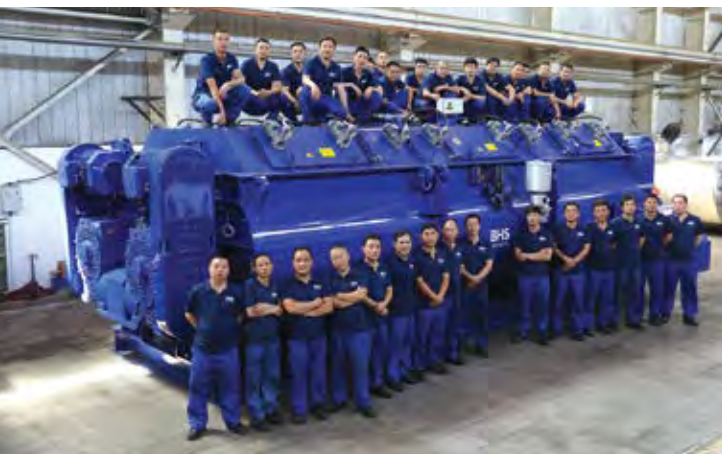
The largest twin-shaft mixer ever built by BHS, with a capacity of 28,000 liters, is completed in August 2019 and installed at a mine in India before 2020. (Photo: BHS-Sonthofen)
