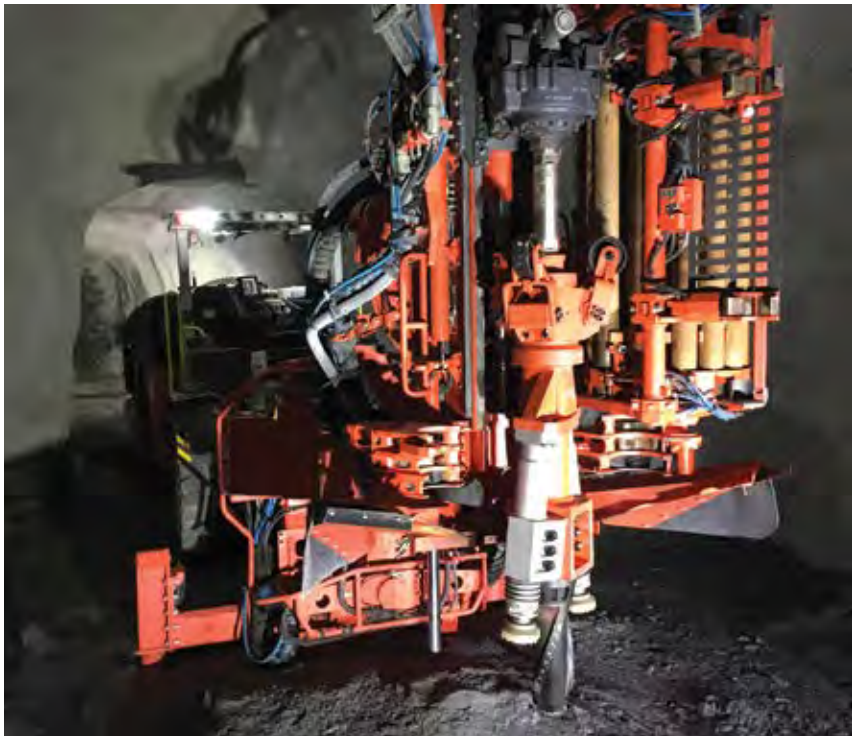
The Sandvik DU412i ITH longhole drill can, without modifications, be used in both production drilling and slot development. Leadership at the company calls it the most versatile rig of its kind on the market. (Photo: Sandvik)
