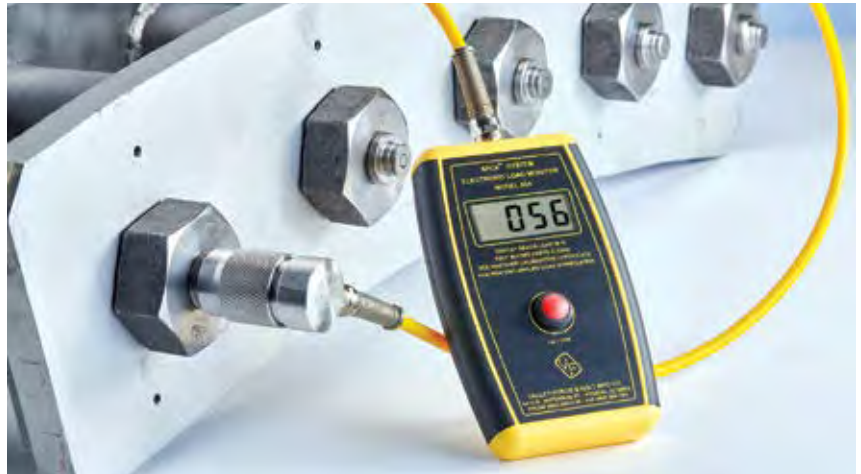
Maintenance technicians can get accurate readings of bolt tension by connecting a digital reader to a datum disk affixed to the end of a Valley Forge fastener.
