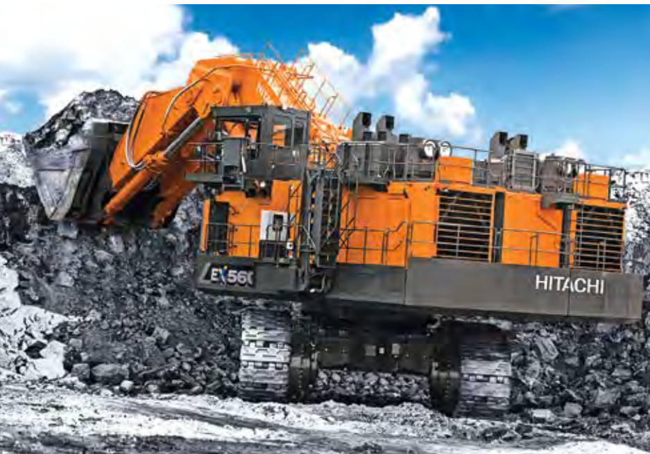
The largest model in Hitachi's new EX-7 Series, the EX5600-7 offers a maximum bucket capacity of almost 45 yd 3 . (Photo: Hitachi)
