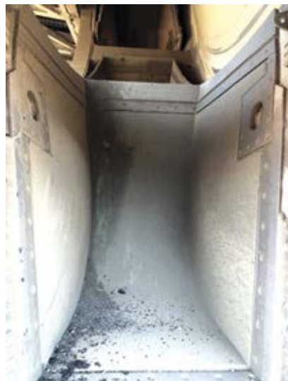
The images above show two mining shovel buckets: one lined with newGEN's PureGRAPH enhanced rubber — known as Armour-GRAPH — and the other with a standard rubber wear liner. The latter shows clear signs of wear at the rear of the bucket.
