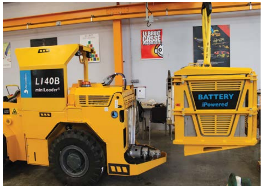
Aramine’s mobile charging station for the miniLoader L140B is equipped with a hydraulic crane.
