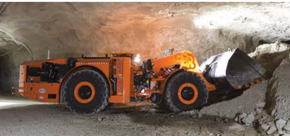
The Joy SR Hybrid LHD's control algorithms optimize efficiencies in applying torque to the ground, controlling wheel slip, and reduces fuel burn.
