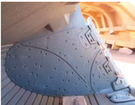
This shovel bucket has been rebuilt with CQMS Razer's PACplate.
