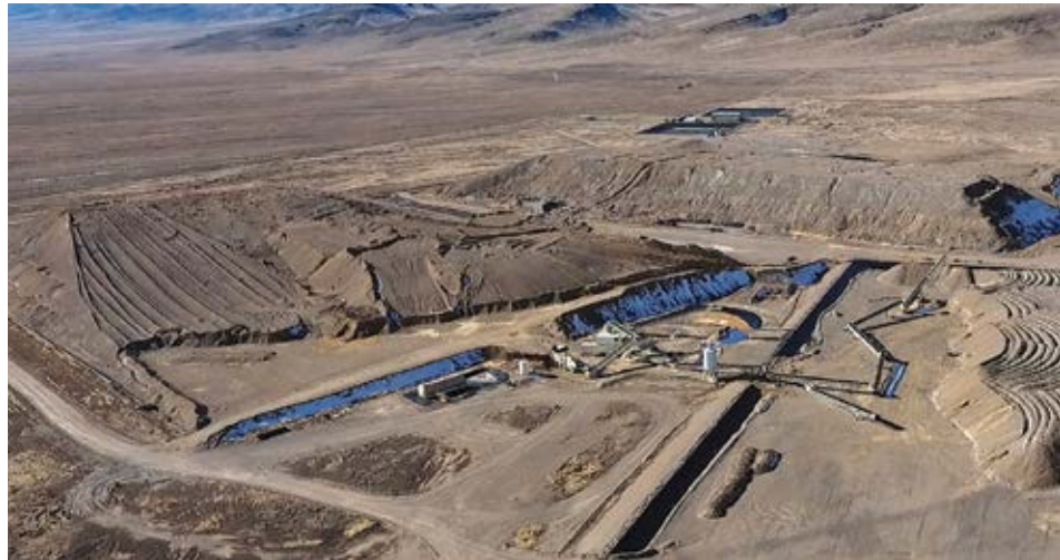
Roughly 150,000 mt of ore had been stockpiled ahead of the crusher at Relief Canyon and was waiting to be placed on the leach pad.
