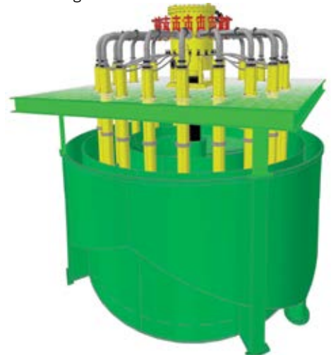
A conceptual sketch of the award winning NovaCell flotation cell. (Photo: Graeme Jameson)
