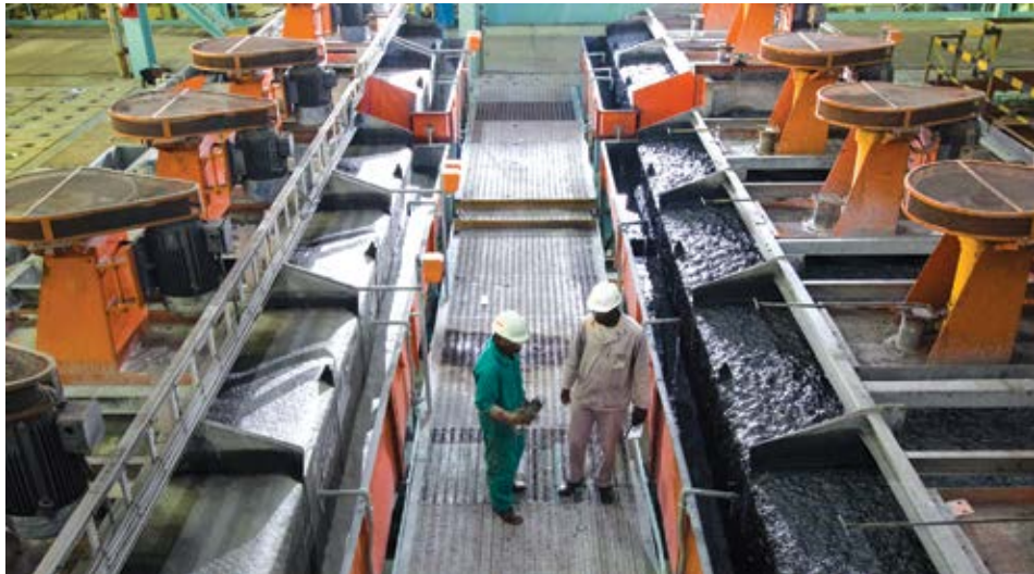
Flotation cells recover copper and cobalt at Katanga Mining's Kamoto concentrator.
