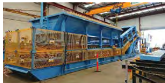
The latest low-profile feeder reclaim hopper under construction by Transmin. (Photo: Bonfiglioli)
