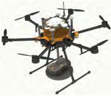
BMT's FED (Flight Enabled Detector) comprises a multirotor drone fitted with the company's Blast Movement Monitor detector.
