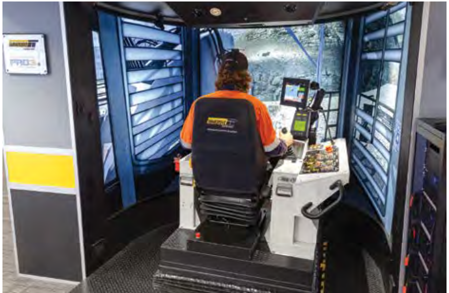
An operator trains on the Cat Command for Hauling system with help from an Immersive Technologies simulator. (Image: Immersive Technologies)
