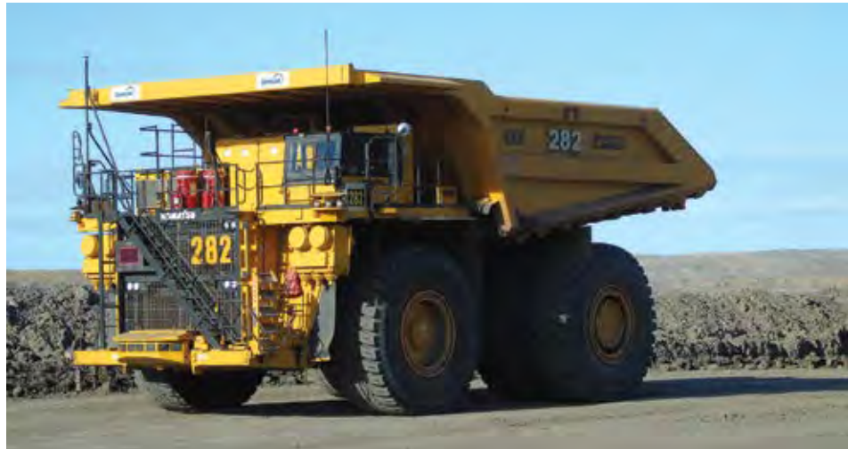
Autonomous haulers need to be fitted with GPS beacons in addition to several other components, such as LiDAR, radar, vehicle controllers, Wi-Fi, etc. (Photo: Suncor)
