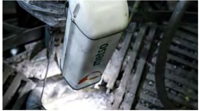
Metso's VisioFroth camera in action. The company says that when used properly, this technology can deliver a 1% increase in recovery grade. (Image: Metso)
