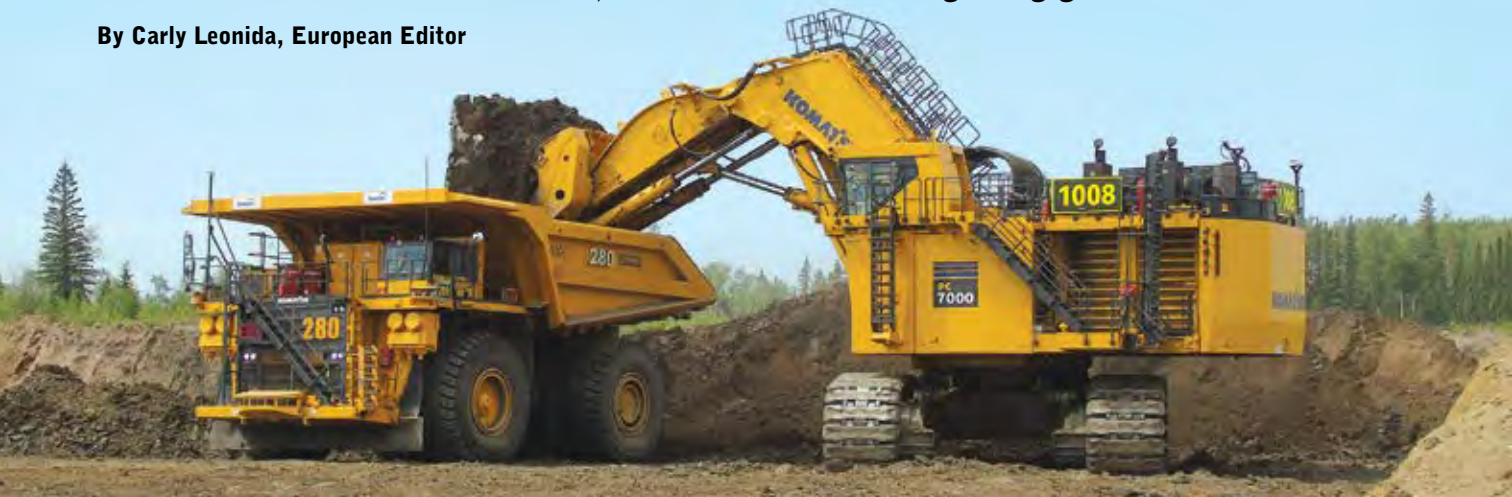
A hydraulic excavator loads an autonomous hauler at Suncor's Steepbank oil sands mine in northern Alberta, Canada. (Photo: Suncor)
