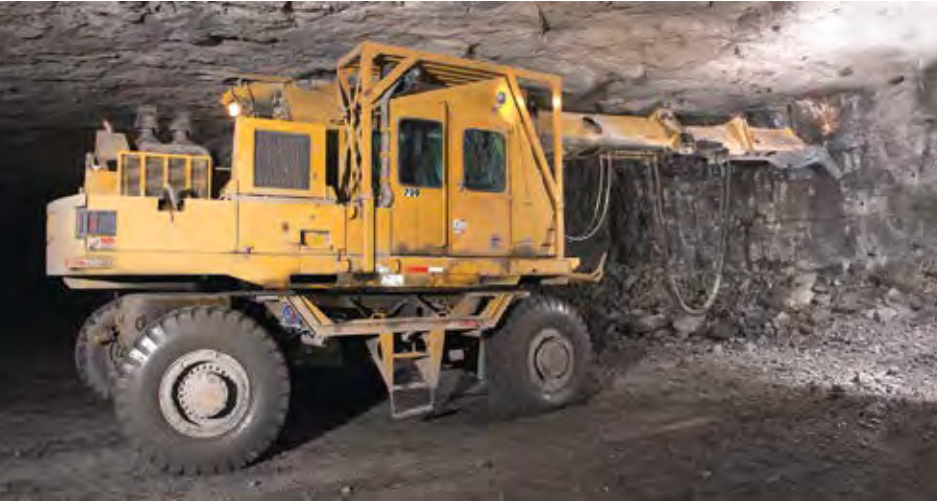
Gradall's scalers feature a boom purpose built for the task. The latest updates to the series include weldments that push machine life out beyond 10,000 hours. (Photo: Gradall)
