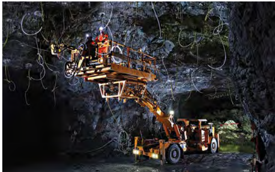
MacLean Engineering's LR3 was built for ventilation fan repair and replacement work, but has graduated to a multipurpose elevated work platform. (Photo: MacLean Engineering)
