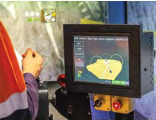
A close-up from the control panel used in the Komatsu Frontrunner AHS. (Image: immersive Technologies)
