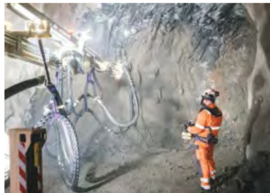
At the 1,000-m level in the Pyhäsalmi mine in Finland, a Normet Spraymec 8100 VC SD is tested. (Photo: Normet)
