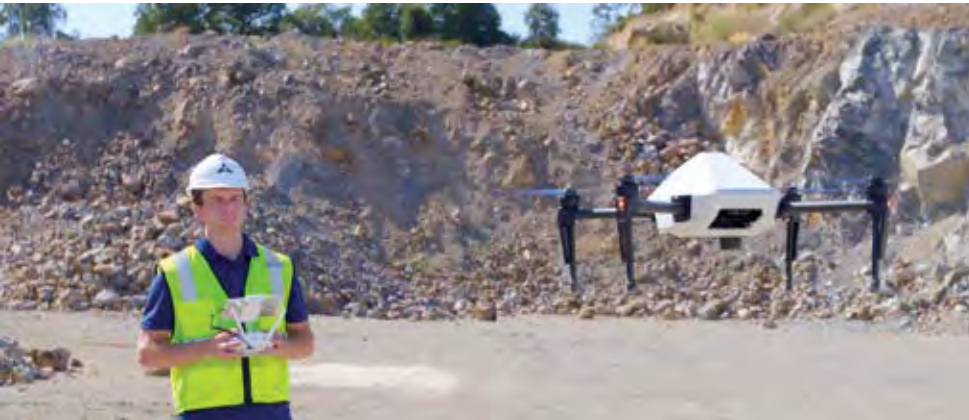
Komatsu has teamed with Skycatch, which specializes in data collection and analysis, to offer an ‘Everyday Drone’ solution for customers interested in performing 3D site surveys. The system is based on Skycatch’s Explore 1 high precision UAV, shown here.
