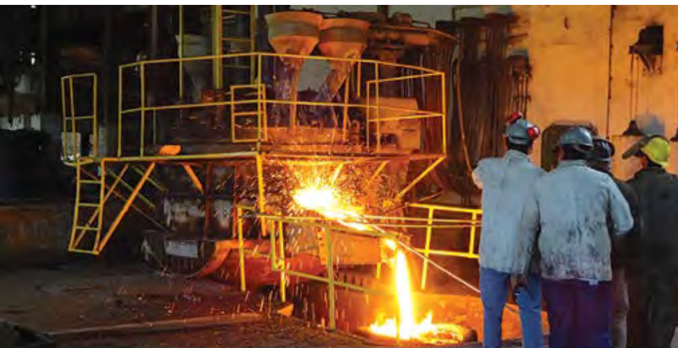
Ferro-nickel metal is smelted and poured at the Horizonte Minerals' Araguaia pilot plant. (Photo: Horizonte Minerals)
