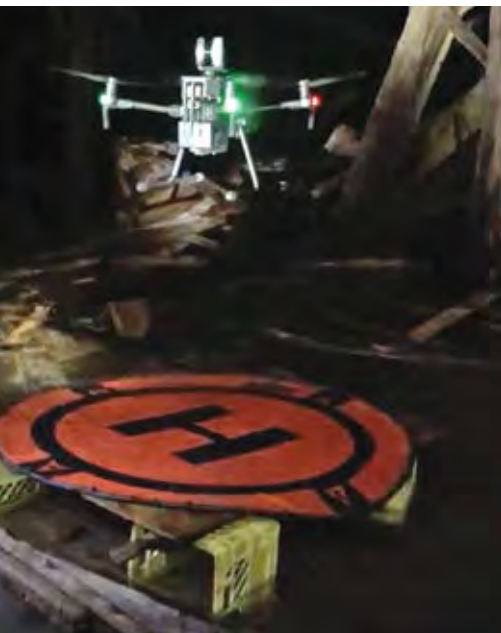
An Exyn A3R drone equipped with a navigational package that allows it to safely avoid obstacles takes off for an underground mine mapping mission.
